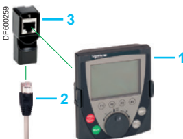
Portable use of the remote graphic terminal: 1 + 2 + 3
