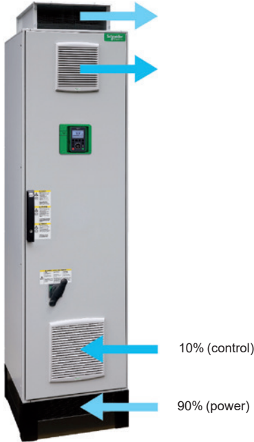
Cooling system with two separate air flows
