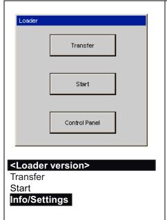
Press the "Transfer" button or use the "Transfer" menu command to set the HMI device to "Transfer" mode
