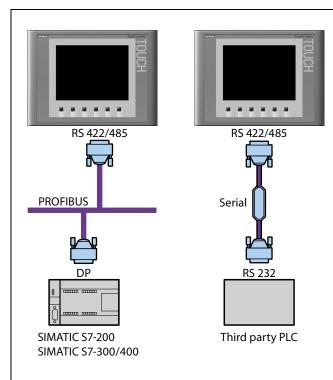
You can connect Basic Panels DP via the RS 422/RS 485 interface to the following SIMATIC PLCs:
