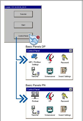
Open the Control Panel by pressing the "Control Panel" button of the Loader.
