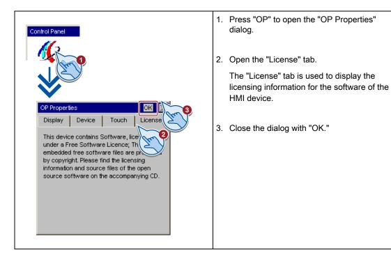
5.1 Configuring devices with graphical Control Panel
