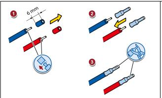
Use power supply cables with a maximum cross-section of 1.5 mm<sup>2</sup>.
