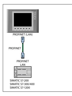
Basic Panels PN can be connected to the following SIMATIC PLCs:
