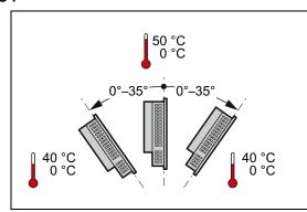
The Basic HMI devices are selfventilating. Vertical and angled mounting is permitted in:
