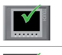
All Basic HMI devices are suitable for horizontal mounting positions.
