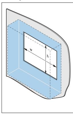
Dimensions of the mounting cutout for the basic HMI devices in horizontal mounting position:
