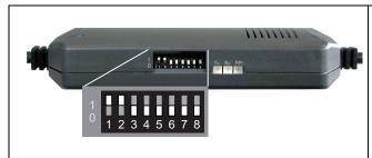
Set the DIP switches 1 to 3 to the same value as in WinCC flexible or WinCC. DIP switches 4 to 8 must be set to "0". In the figure, the bit rate is set to 115.2 kbps.
