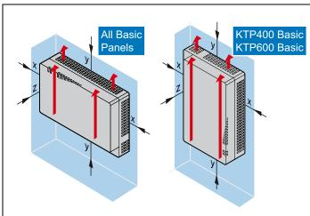
Required clearance around the HMI devices.
