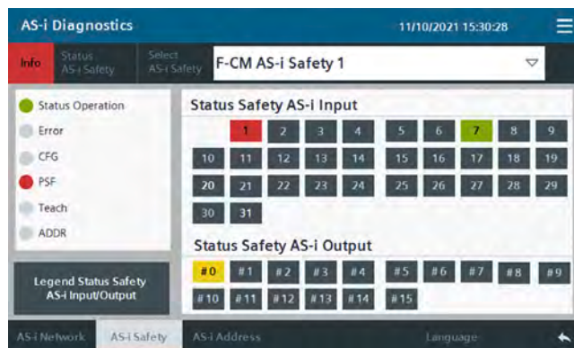
Diagnostics block for F-CM AS-i Safety ST
