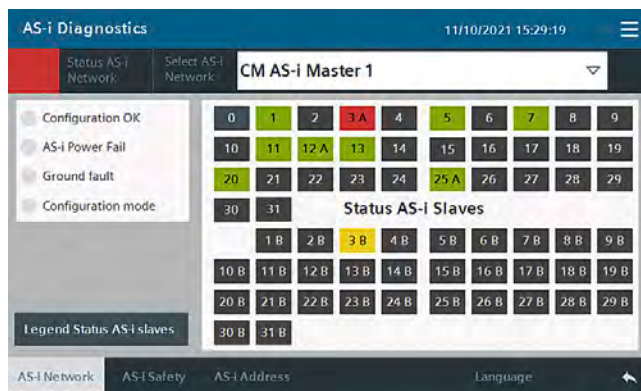
Diagnostic block for CM AS-i Master ST
