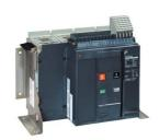
Circuit breaker frame, MasterPact NT16H1, 1600A, 42kA/440VAC 50/60Hz (Icu), 4 poles, fixed, without control unit
