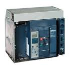
Circuit breaker frame, MasterPact NT16H2, 1600A, 50kA/440VAC 50/60Hz (Icu), 4 poles, drawout, without control unit
