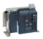
Circuit breaker frame, MasterPact NW20N1, 2000A, 42kA/440VAC 50/60Hz (Icu), 4 poles, fixed, without control unit
